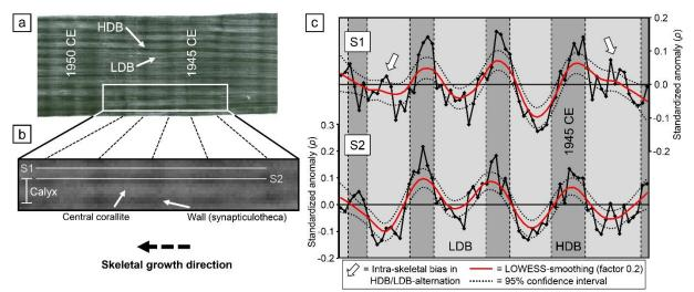
(a) Coral X-ray image, (b) gamma densitometer scan pattern with measured sections (S1: central corallite, S2: thecal wall), (c) skeletal density ( $\rho$ ) of both sections as trend-less standardized anomalies.
