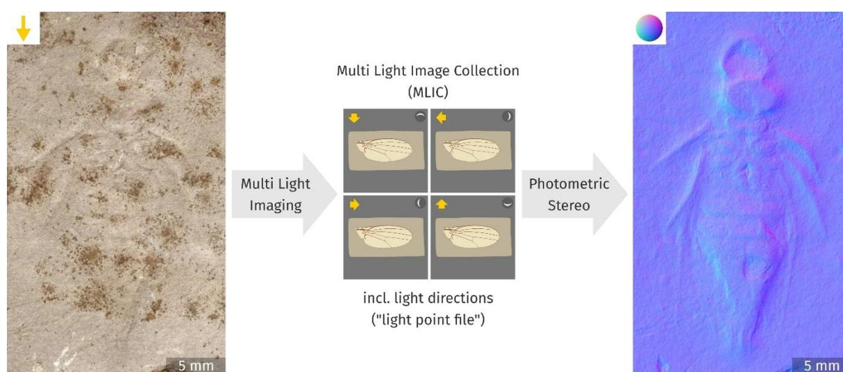
High level overview of a Multi Light Imaging workflow: capturing multiple images with different illumination settings (left side), processing using Photometric Stereo and visualization in form of normal maps (right side).
